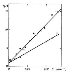
Fig. 2. Dependence of  $\varphi_0/\varphi$  on quencher concentration for added naphthalene ( $\Box$ ) and copolymers VPK/2VN ( $\bullet$ ) in polymer film (line 1) and ( $\triangle$ ) in solution at concentration 12 g/l (line 2).
