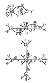
Fig. 1. Schematic representation of the bonding models for some halogen—copper compounds.
