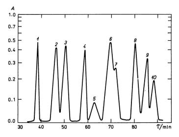
Fig. 2. Separation of a standard mixture of amino acids containing selenolanthionine in a catex column  $(62 \times 0.8 \text{ cm})$  eluted with a pH 3.25 buffer.
