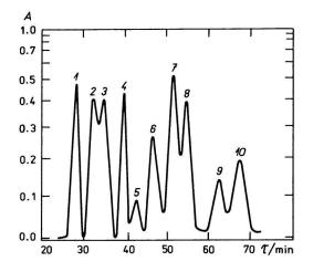
Fig. 1. Separation of a standard mixture of amino acids containing selenolanthionine on a catex column  $(37 \times 0.8 \text{ cm})$  eluted with a pH 3.25 buffer.
