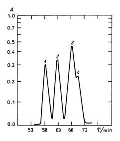
Fig. 3. Record of the separation of lanthionine and selenolanthionine on a 62 cm long catex column eluted with a pH 3.25 buffer.
