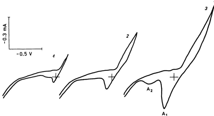
Fig. 2. Cyclic-voltammetric records of deposition and dissolution of lead and aluminium in ethylbenzene electrolyte for various switching potential values at scan rate 0.0166 \text{ V s}^{-1} . c(\text{AlBr}_3) = 1.82 \text{ mol dm}^{-3} ; c(\text{KBr}) = 0.8 \text{ mol dm}^{-3} ; c(\text{PbBr}_2) = 8.65 \times 10^{-3} \text{ mol dm}^{-3} . Switching potential E_s : 1. — 0.2 \text{ V} ; 2. — 0.4 \text{ V} ; 3. — 0.6 \text{ V} .
