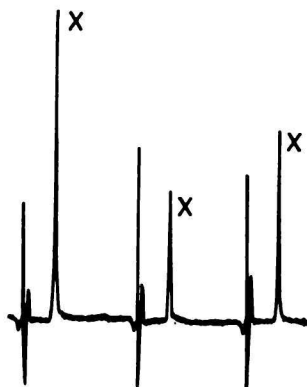
Fig. 2. Chromatogram of three injections of the same solution of chlorhexidine (X) dissolved in methanol ( c = 0.0319 \text{ mol m}^{-3} ).
