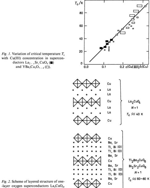
Tl<sub>2</sub>Ba<sub>2</sub>CuO<sub>6</sub>, and Bi<sub>2</sub>Sr<sub>2</sub>CuO<sub>6</sub>.
