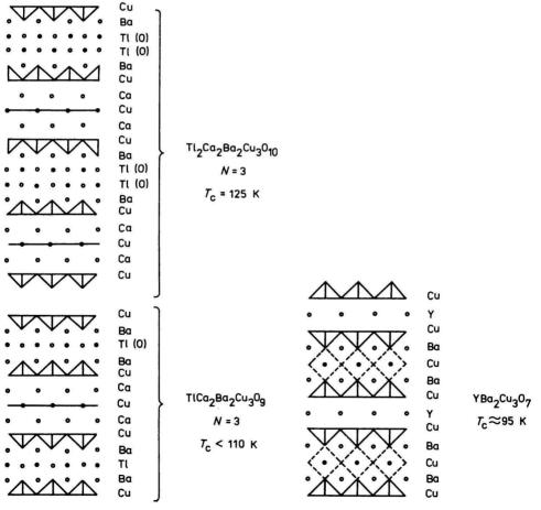
Fig. 4. Scheme of layered structure of threelayer oxygen superconductors  $Tl_2Ca_2Ba_2Cu_3O_{10}$ and  $TlCa_2Ba_2Cu_3O_9$ .
