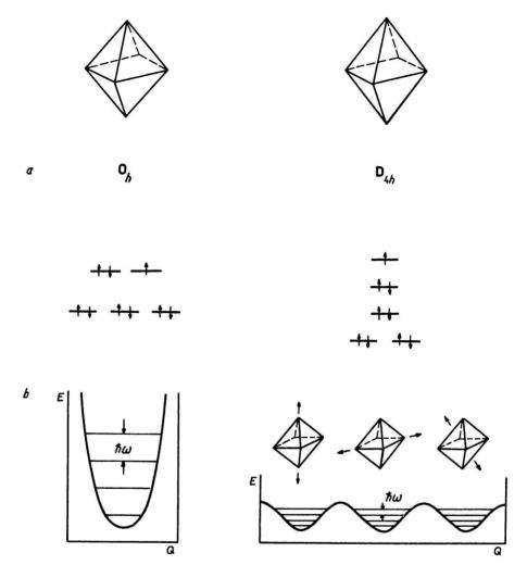
Fig. 8. Scheme of the Jahn—Teller distortion in the octahedral Cu(II) complex. a) Degenerate levels and removement of degeneration in the configuration of expanded tetragonal bipyramid; b) shape of adiabatic potential with the scheme of distortion of the octahedron in individual minima and the scheme of vibrational levels.
