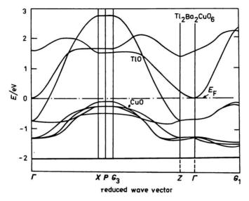
Fig. 9. Energy spectrum of band structure of the system  $Tl_2Ba_2CuO_6$  as a function of the reduced wave vector.
