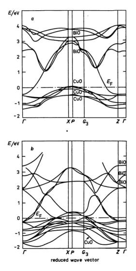
*Fig. 10.* Energy spectrum of band structure of the system Bi<sub>2</sub>Sr<sub>2</sub>CaCu<sub>2</sub>O<sub>8</sub>. *a*) Ideal crystal structure; *b*) structure with model introduction of oxygen vacancies.
