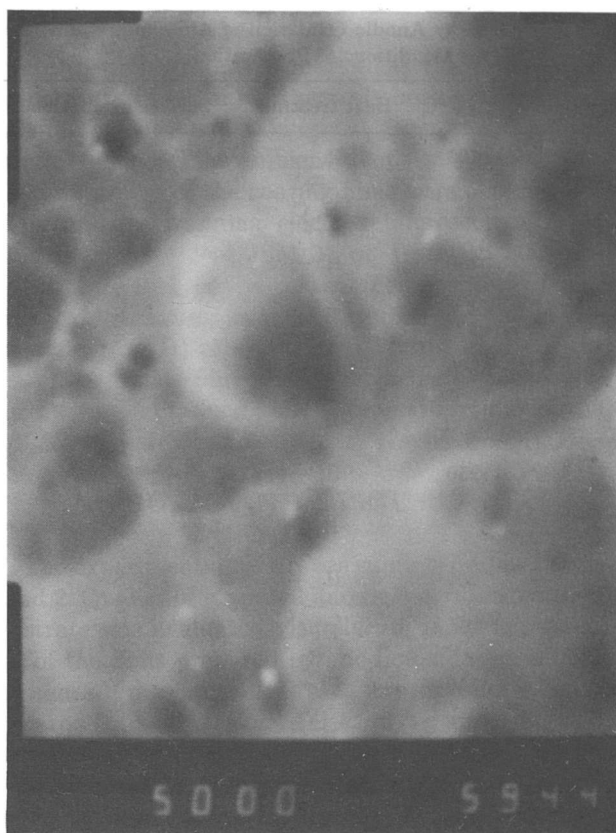
Fig. 4. Microstructure of surface coating without shrinkage for 20 min anodic oxidation and temperature of calcination for the sol-gel process of 250°C ( \times 5000 magn.).
