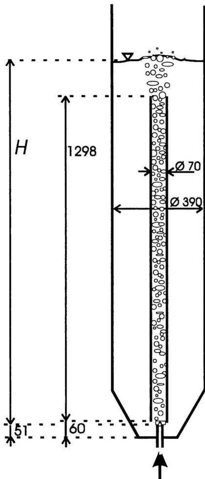
Fig. 1. Laboratory model 1 12 of the pachuca (dimensions/mm).
