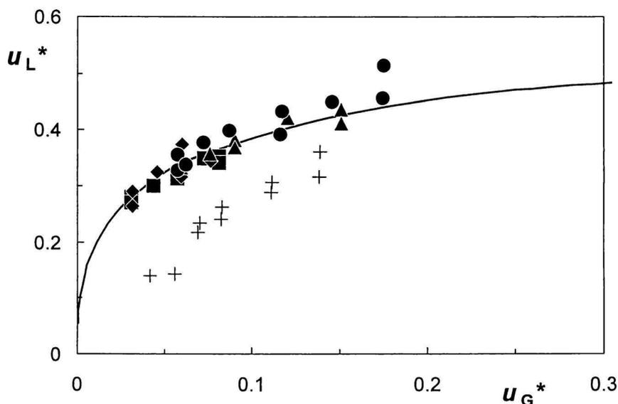
Fig. 3. Dimensionless superficial velocity of liquid as a function of gas superficial velocity for particular values  $H$ . The values are normalized employing  $\zeta = 4.5$ . ■  $H = 1525$  mm; ◆  $H = 1471$  mm; ▲  $H = 1417$  mm; ●  $H = 1307$  mm; +  $H = 1180$  mm; —  $B = 0.005$ .
