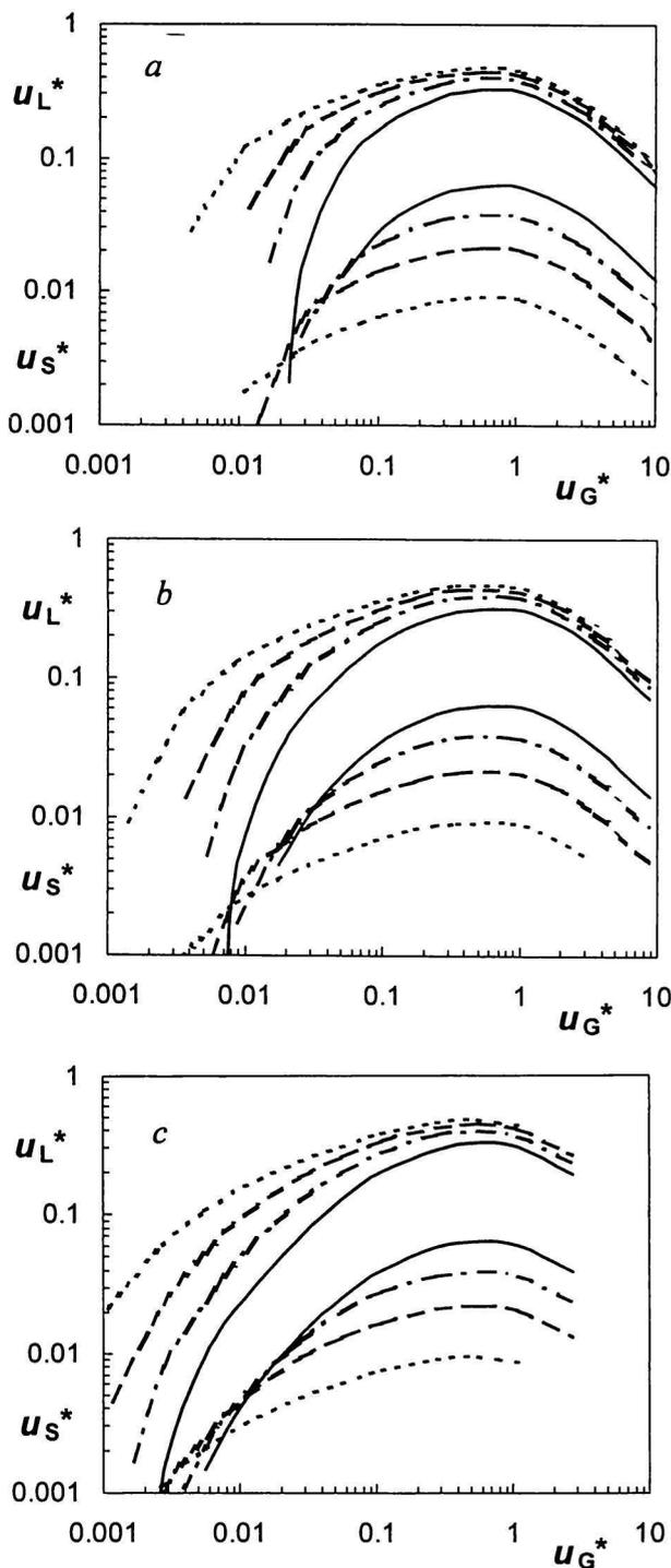
Fig. 4. Dimensionless superficial velocities of liquid and solid as a function of gas flow rate for  $s = 2.75$ . Three plots are for different  $B$ , a)  $B = 0.01$ , b)  $B = 0.001$ , c)  $B = 0.0001$ . Upper group of curves for different  $X$  belongs to  $u_L^*$ , lower group belongs to  $u_S^*$ . ----  $X = 0.02$ ; ----  $X = 0.05$ ; - · - · -  $X = 0.10$ ; —  $X = 0.20$ .
