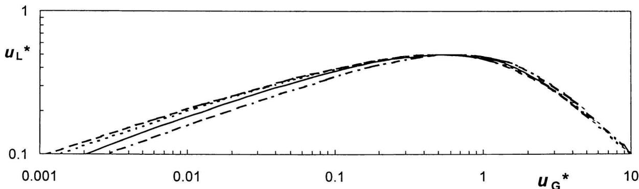
Fig. 2. Dimensionless superficial velocity of liquid as a function of gas superficial velocity for particular values of the parameter  $B$ . - · - · -  $B = 0.1$ ; —  $B = 0.01$ ; - - -  $B = 0.001$ ; - - - -  $B = 0.0001$ .
