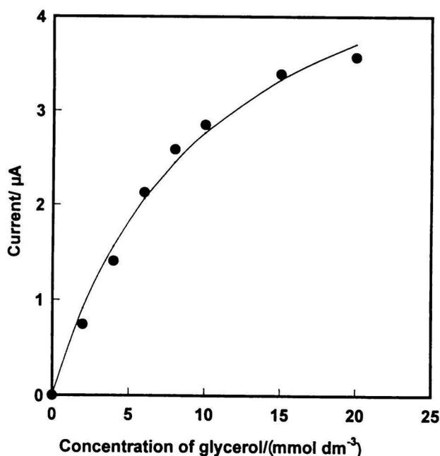
Fig. 1. Calibration graph of the glycerol biosensor in 0.05 mol dm<sup>-3</sup> sodium acetate buffer (pH = 6).
