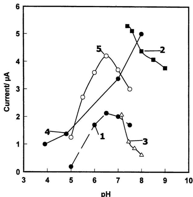
Fig. 3. Dependence of the response of the glycerol biosensor on pH in different buffer solutions. The glycerol concentration was  $5 \text{ mmol dm}^{-3}$  (1. phosphate buffer, 2. borate buffer, 3. tris-malate buffer, 4. glycine buffer, 5. acetate buffer).
