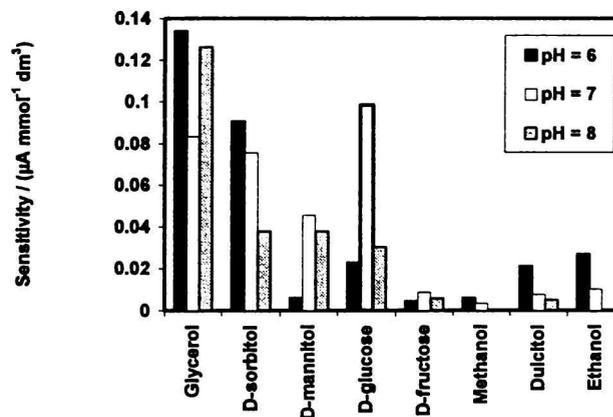
Fig. 2. Response of the *Gluconobacter* sp. membrane-based biosensor to various substrates. The sensitivity was measured in three buffer solutions: acetate, pH 6, phosphate, pH 7, and glycine, pH 8.
